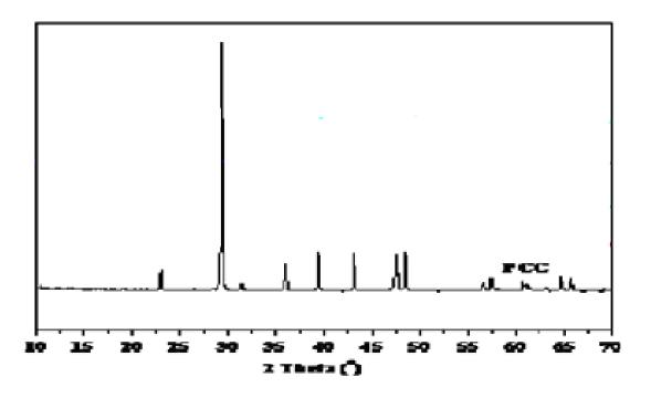
Figure 1: XRD pattern Precipitated calsium Carbonate.
